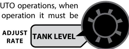
**ALARM ENABLE:** Selecting the RATE position on page three (3) allows the user to turn the audible ALARM ENABLE On or Off by using the adjustment of the “+” or “-” (Reset) keys. Setting ALARM ENABLE to Off will disable all audible Alarms under all conditions.
