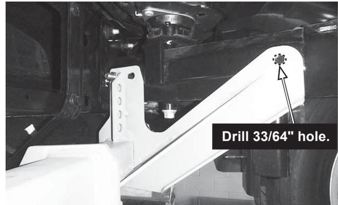
7. Locate the 1/2" x 1-1/4" cap screws with 18" handles. Insert the cap screw handles into the frame and insert the cap screws through the holes drilled in Step 6. Install 1/2" locknuts on the cap screws and finger tighten.
