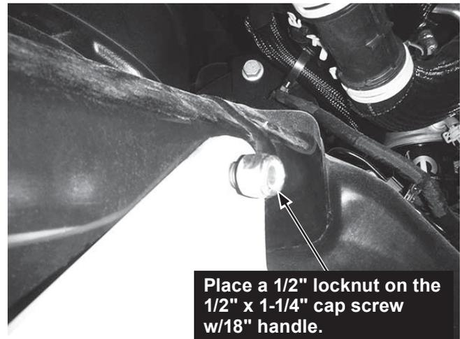
8. Using the remaining slotted holes as guides, drill 33/64" holes through the frame.
