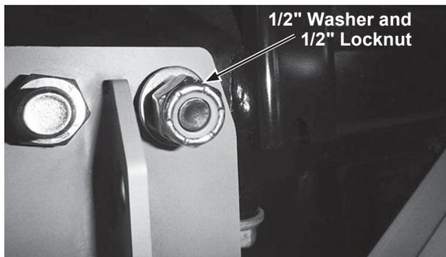
10. Tighten all fasteners according to the torque chart.
