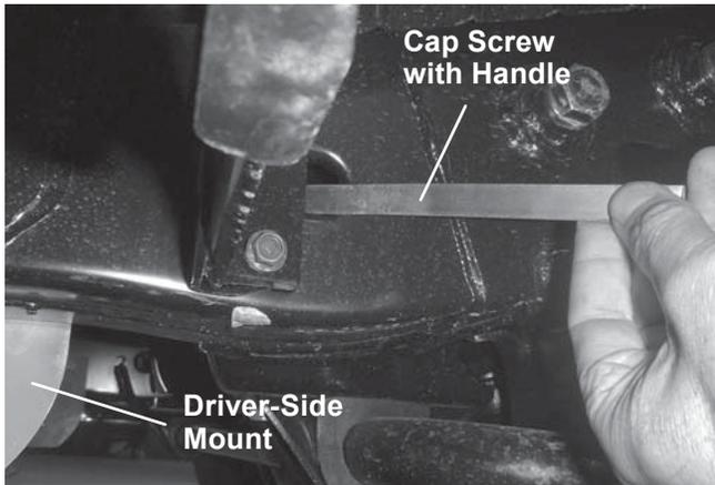
11. Insert a 1/2" x 1-1/2" cap screw with handle into the access hole on the inside of the driver-side frame at the location shown. Insert the cap screw through the front hole drilled in Step 7 and the hole in the front tab of the mount. Install a 1/2" locknut onto the cap screw and hand tighten.
