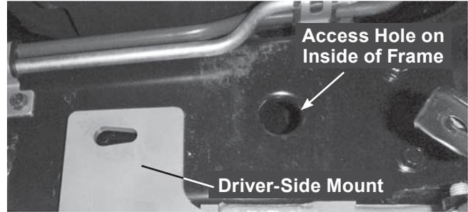
12. On the passenger's side of the vehicle, insert a 1/2" x 1-1/2" cap screw with handle into the access hole to the rear of the mount on the inside of the vehicle frame in the location shown. Insert the cap screw through the rear 17/32" hole drilled in Step 8 and the rear slot on the mount. Place a 1/2" washer onto the cap screw, install a 1/2" locknut, and hand tighten.
