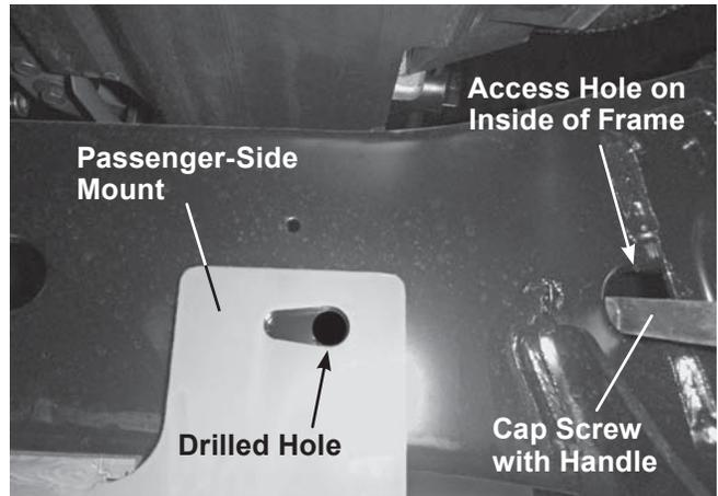
13. Insert a 1/2" x 1-1/2" cap screw with handle into the access hole shown on the inside of the passenger-side vehicle frame. Insert the cap screw through the front 17/32" hole drilled in Step 8 and the hole in the front tab of the mount. Install a 1/2" locknut onto the cap screw and hand tighten.
