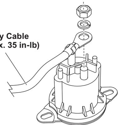
**NOTE:** Use dielectric grease on all electrical connections to prevent corrosion. Fill receptacles and lightly coat ring terminals before assembly.
