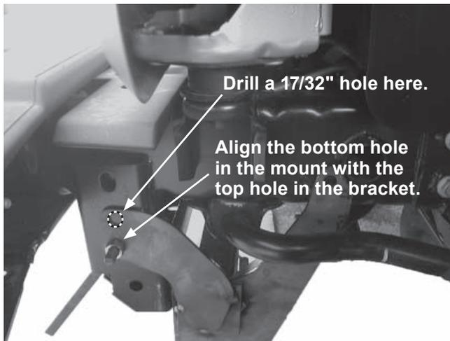
**NOTE: Front wheels should be straight ahead for easiest installation.**
