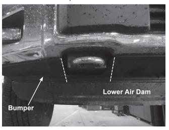
2. Remove the front tow hook fasteners and loosen the rear fasteners. Remove the tow hooks by sliding them forward and then downward. Leave the rear fastener in position as shown.
