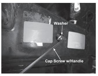
8. Secure the other side of the frame rail with a washer and locknut as shown. Hand tighten the fasteners so that the mount tab comes just into contact with the frame rail. Do not fully tighten at this time. Repeat steps 7 and 8 on the driver's side of the frame rail.
