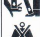
Blade could drop unexpectedly, crushing or trapping limbs. Lower blade when vehicle is parked.
