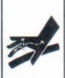
To prevent serious injury or death: Relieve pressure on hydraulic system before servicing or disconnecting. Wear proper hand and eye protection when searching for leaks. Use wood or
