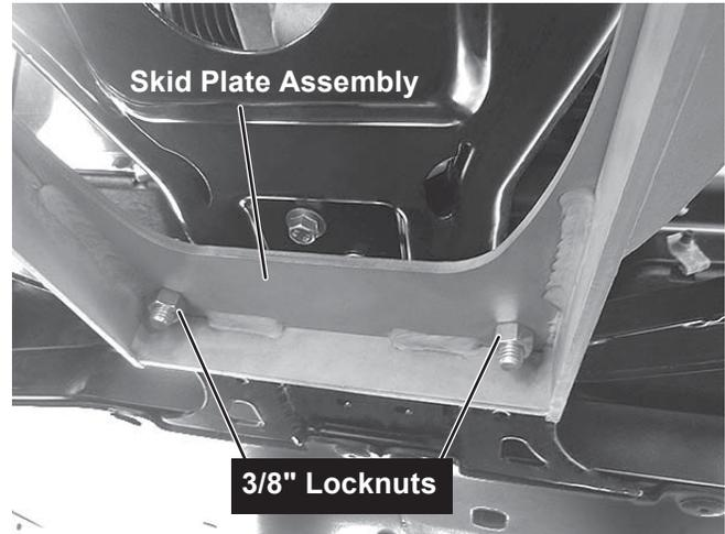
6. Install 3/8" washers on two 3/8" x 1-1/4" cap screws. Insert the cap screws with washers through the slots on the front of the vehicle.
