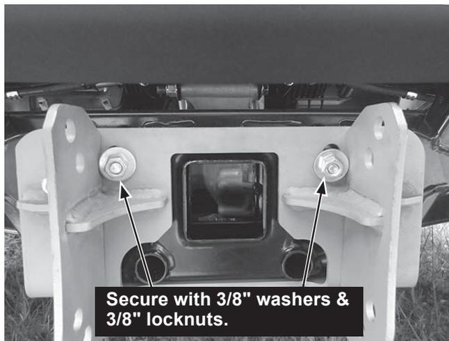
7. Install two 3/8" x 1-1/4" cap screws down through the holes enlarged in Step 2. Secure with 3/8" locknuts. Hand tighten the locknuts.
