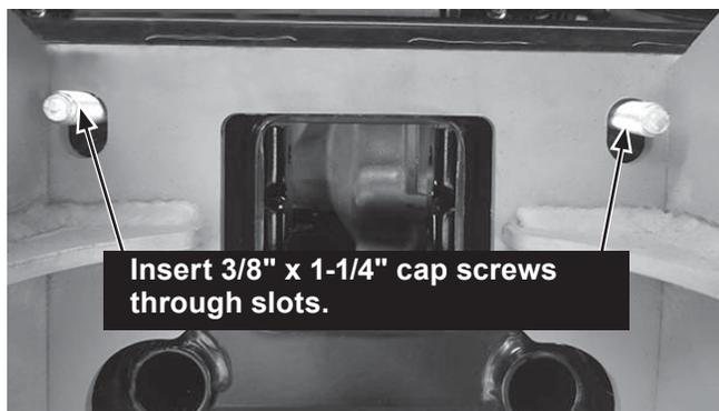
Secure cap screws with 3/8" washers and 3/8" locknuts. Hand tighten the fasteners.
