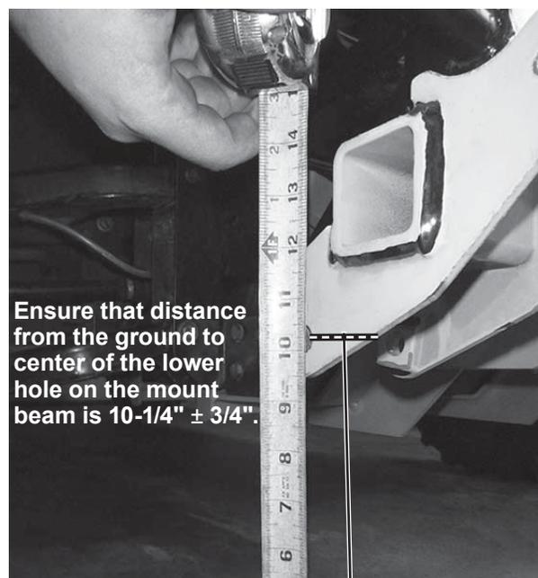
10. Measure the distance between the mount beam rear hole and the ground. If it exceeds 11-1/2", install the accessory Height Adapter Plate Kit (PN 77555) to ensure optimum plowing performance.
