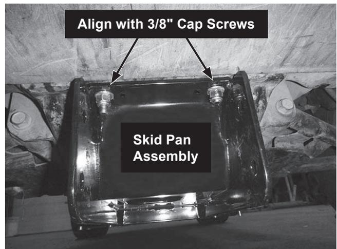
4. Place U-bolt shim plates in position on the top side of the skid pan assembly. Position two U-bolts on each side of the mount (four total), as shown. Check that the U-bolts have at least 1/4" clearance from any other vehicle components. Adjust the position forward or aft, as needed. Secure with 3/8" washers and locknuts.
