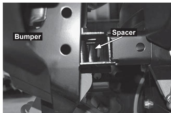
4. Place the driver-side hanger in position against the bottom of the bumper so that the 7/16" x 2-1/2" cap screws pass through the hanger holes. Secure with 7/16" locknuts and repeat on the passenger's side.
