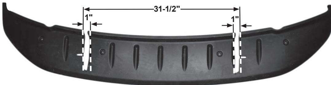
Cut slots in air dam as shown.
