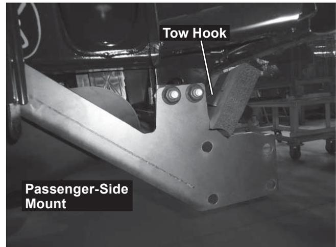
Reuse the tow hook fasteners to loosely secure the mount. Do not tighten fasteners at this time.
