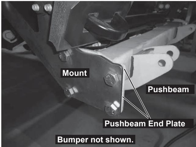
5. Measure the distance between the pushbeam rear hole and the ground. If it exceeds 11-1/2", install the accessory Height Adapter Plate Kit (PN 77555) to ensure optimum plowing performance.
