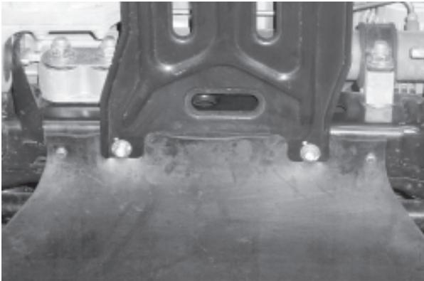
**If the vehicle is not equipped with a transaxle skid plate**, align the holes in the rear splash shield retainer and the tapered end of the splash shield with those in the vehicle frame cross member. Install two M6 x 1.00 cap screws and flat washers (supplied with the mount) through the rear splash shield retainer and splash shield and into the cross member. Do not over tighten.
