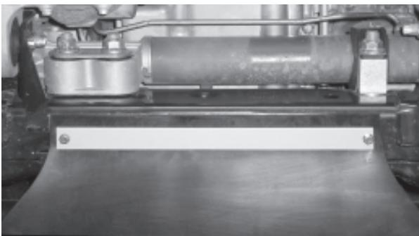
5. Make sure the splash shield is under the vehicle sway bar, then pull the uncut end of the shield to the vehicle bumper support beam.
