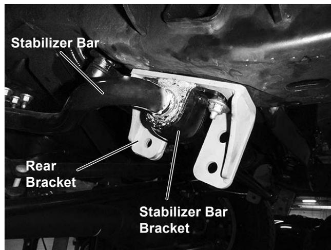
8. Position the passenger-side mount as shown. Insert two 1/2" x 2" cap screws through the mount holes against the inner frame surface. Secure with 1/2" locknuts and 1/2" washers on the inside of the frame.
