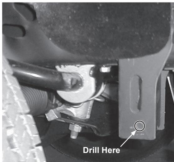
7. Align the thrust arm's 1/2" diameter holes with these drilled holes and loosely secure with a 1/2" x 1-1/4" cap screw and locknut. Align the 1/2" diameter hole on the opposite end of the thrust arm with the 1/2" diameter hole on the rear of the front mount. Loosely secure with a 1/2" x 1-1/4" cap screw and locknut. Place a 3/8" cap screw through the smaller holes of the thrust arm and front mount and loosely secure with 3/8" locknut.
